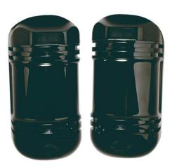
The DS422i and DS426i are dual-beam photoelectric detectors designed for indoor and outdoor applications. Consisting of a separate transmitter and receiver, they are designed to activate an alarm when an intruder passes within the direct line of sight between the transmitter and receiver.
