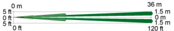
Top View Optional Long Range Coverage: 25 m to 36 m x 3 m (80 ft to 120 ft x 10 ft)
