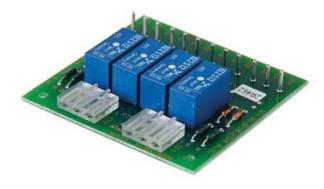
Panel relay module RTP with four relays, each relay with a double-throw contact for potential-free outputs, up to six RTPs can be plugged into AVM.
