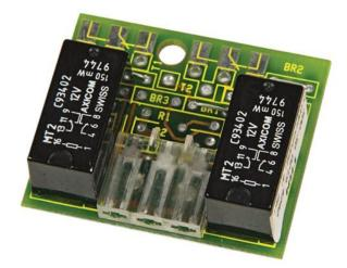
Panel relay module TRN with two relays, each relay with a double-throw contact for potential-free outputs. The AVM 100 can be extended with up to six TRNs.
