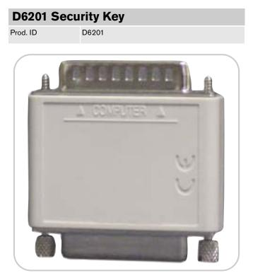
The D6201 Security Key is designed for use with a parallel port.
