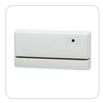
The DS1109i Detector uses microprocessor-based Sound Analysis Technology (SAT) to listen for the specific frequencies associated with breaking glass. It can be used to detect breakage of plate, tempered, laminated and wired glass types. A built-in environmental test feature alerts the installer of false alarm hazards in harsh environments. It is specially designed to be mounted on door or window frames, too. A built-in magnetic contact allows monitoring of a door or window opening.
