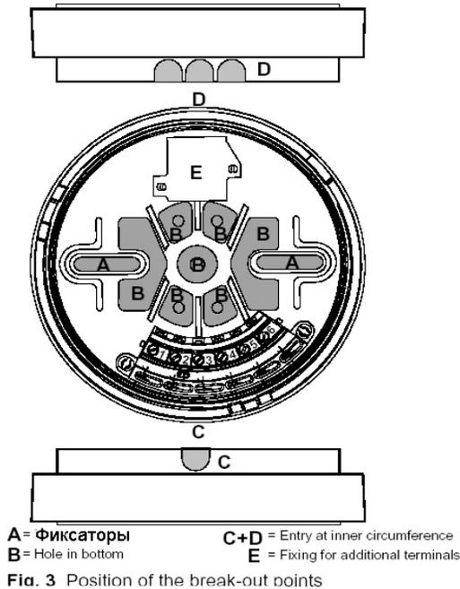
Fig. 3 Position of the break-out points
