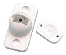
Surface mount the plastic low profile bracket on a wall for mounting various types of detectors. The vertical pivot range is +10° to -20°; the horizontal pivot range is ±25°.
