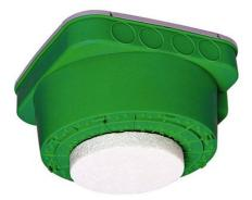
FAA-500-CB built-in housings are used to install 500 and 520 series detectors in concrete ceilings. These make it possible to position cable ducts with ease and precision. A ceiling mount back box is installed in the built-in housing which receives the base and the detector.
