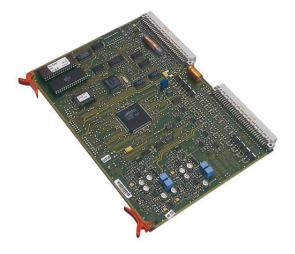
For additional connection of up to 4 loop or 8 stub lines
