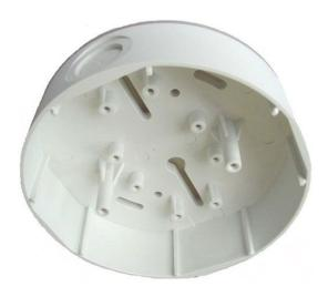
The additional base MSC 420 was conceived specially for surface-mounted cable feeds with cable protection conduits and has 2 opposing pre-cut inlets of 20 mm diameter and 2 additional opposing and prepared inlets for up to 28 mm diameter.
