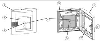
In the event of an alarm, the glass pane (2) is broken first, then the manual call point (3) is pressed hard.
