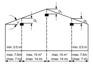
D<sub>H</sub> Horizontal distance between detector and wall: 0.5 m to 7.5 m (VdS max. 7.0 m)
