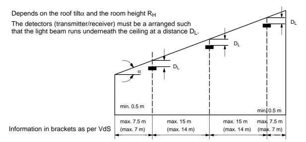
D<sub>H</sub> Horizontal distance between detector and wall: 0.5 m to 7.5 m (VdS max. 7.0 m)
