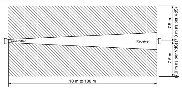
**Note:** Since smoke above the source of a fire does not just rise vertically upwards, but spreads out in a mushroom-like shape (depending on air currents and any air cushions present), the width of the monitoring area is considerably greater than the diameter of the IR beam.
