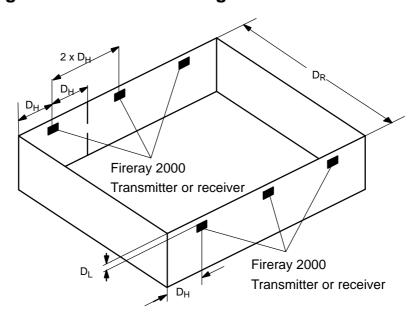
D<sub>H</sub> horizontal distance between detector and wall: 0.5 m to 7.5 m (VdS max. 7.0 m)
