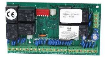
The DX3010 Octo-output Expander connects directly to the data bus of a compatible control panel. Each expander adds eight fully programmable Form C relay outputs. Each output operates individually from the other seven outputs for complete flexibility. Install up to three expanders in a control panel enclosure.
