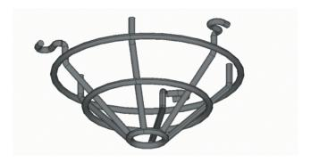
In the case of installation of the detector e.g. in a sports hall, the protective basket prevents balls or other sports equipment hitting and possibly damaging the detector. The robust protective basket consists of 5 mm round steel, and is painted aluminum gray (RAL 9007).
